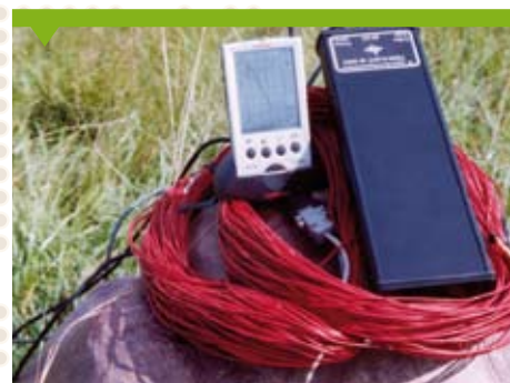
TDEM: equipment used to localize the saline water intrusion Sri Lanka-2006
