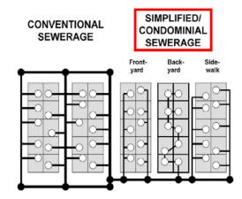
while in the case of water they are generally located under sidewalks to allow for individual metering. This design permits the adaptation of the network to local topographic conditions and different urbanization patterns.
