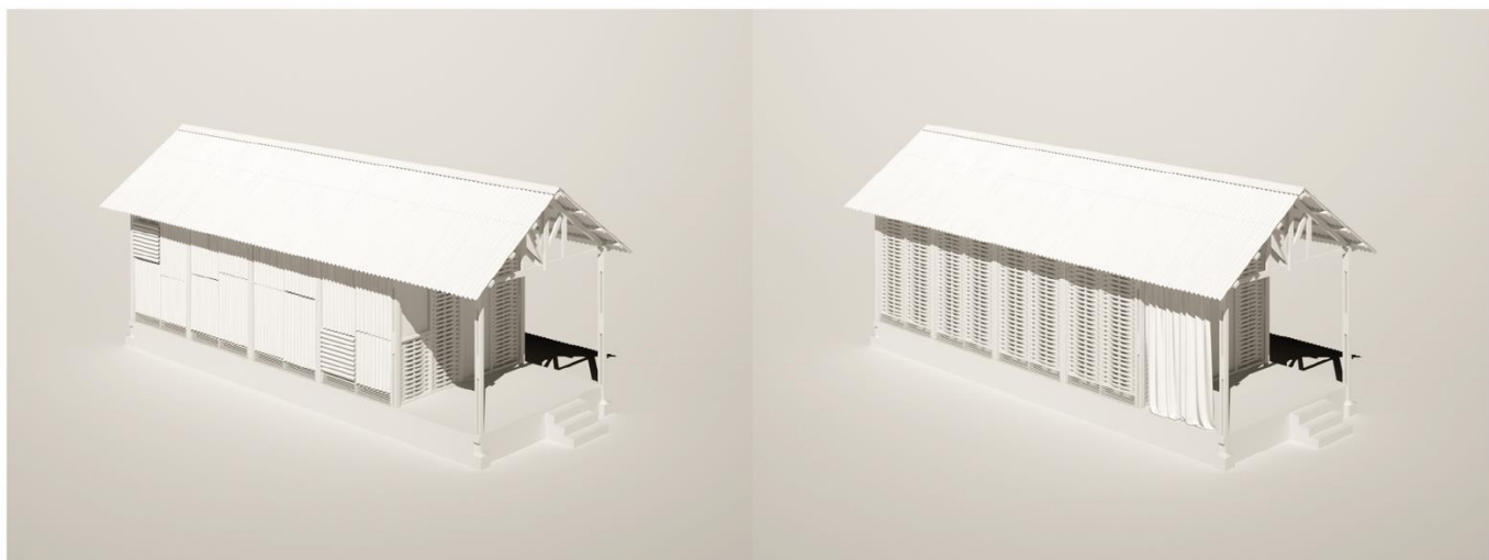
c. metal sheets to cover clissage walls
