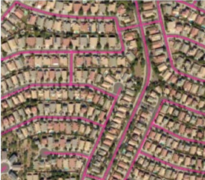
Figure 35: In this neighbourhood in Phoenix, Arizona, 4-way intersections are uncommon, harming walkability and increasing travel distances.
