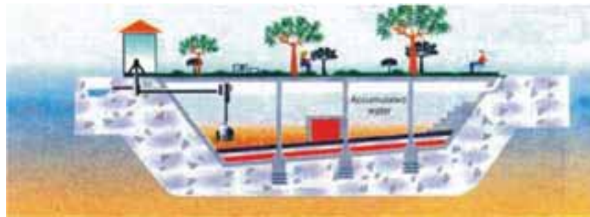
Figure 3.34. Covered detention system (DAEE)
