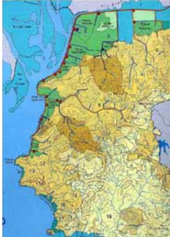
Figure 6.11. City of Porto Alegre bordering on the Jacuí delta and lake Guaíba. Runoff from the green areas is pumped into lake Guaíba when the dyke protects them from flooding. Runoff from the brown areas takes place by gravity and in conduits under pressure.
