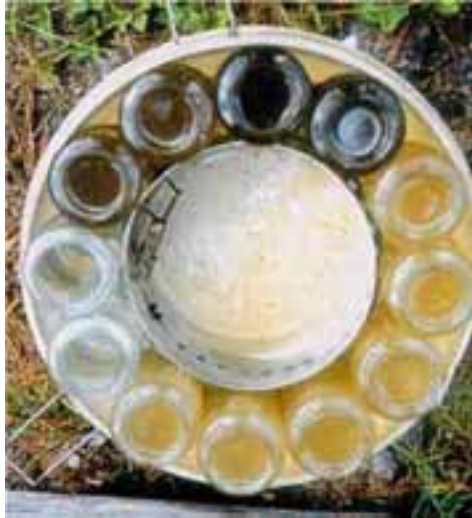
Figure 3.12. Samples of storm water quality The brown bottle (at 9 o'clock) corresponds to the onset of precipitation.
