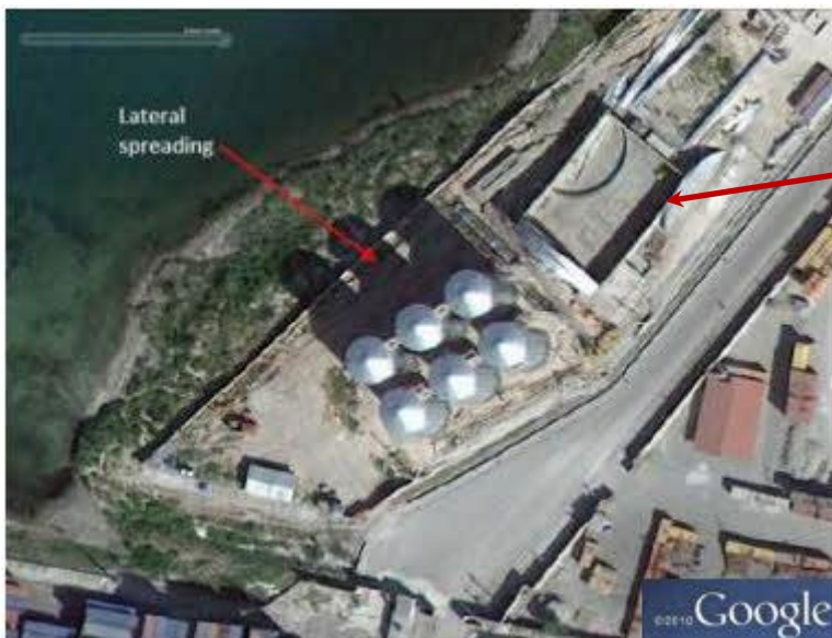
Figure 4.18: Lateral spreading behind the silo structures
