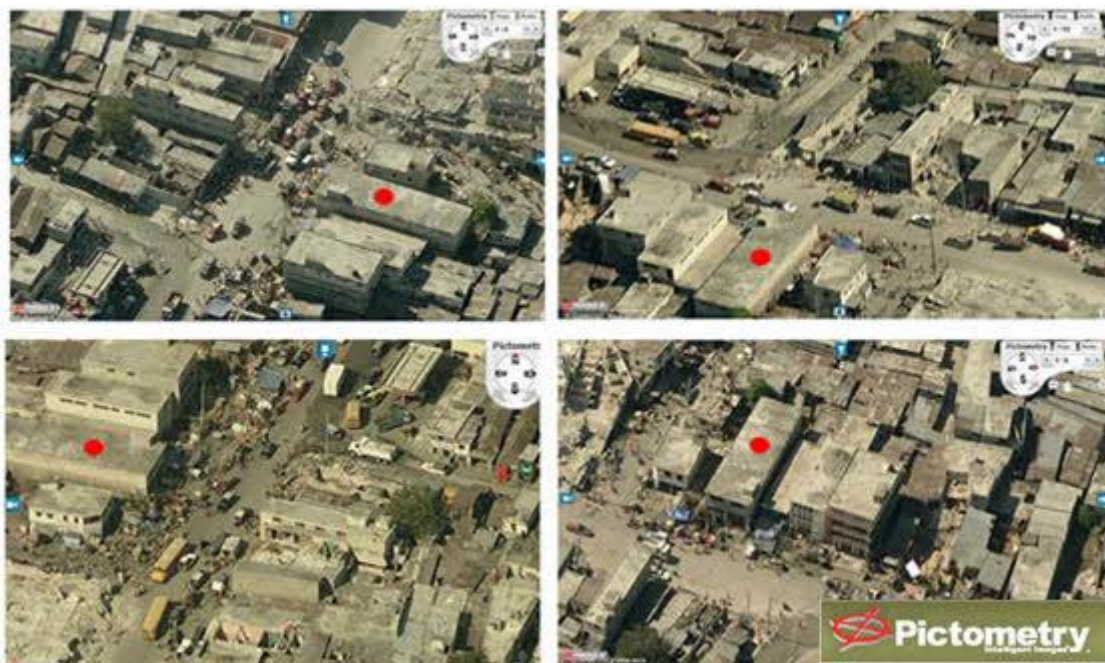
Figure 6.2: A set of Pictometry oblique aerial images for a commercial area in Port-au-Prince. A red spot is placed on the same building in the four directional images.
