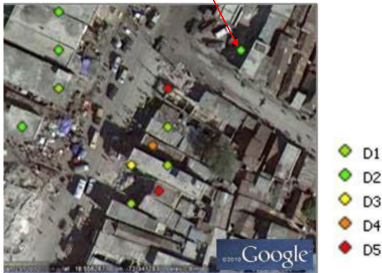
Figure 6.9: The buildings and their damage grades assigned by the EEFIT team.
