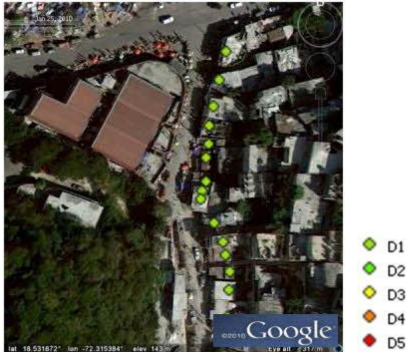
Figure 6.16: Overview of location 17 where all buildings were assigned D1 by the EEFIT team.
