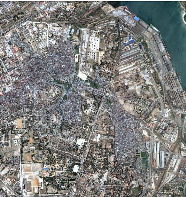
Above: Colour orthophoto (60cm resolution) of Dar es Salaam, Tanzania. Dense and complex structure of unplanned housing is clearly distinguishable from planned residential and industrial development. Individual buildings can be identified and counted.
