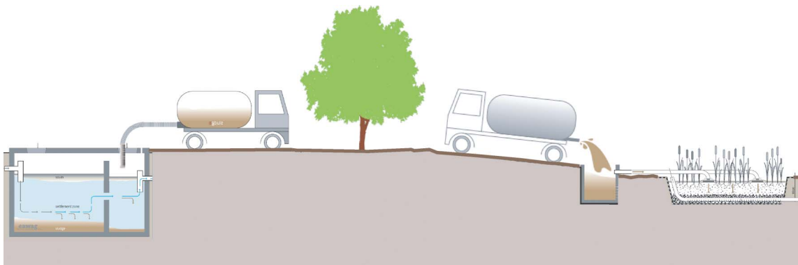
Figure 3. HCES consider the entire sanitation system and a variety of technical options that are available from the toilet to the final treatment. Example of a sanitation system configuration involving storage (septic tank), transport (motorised emptying) and treatment (constructed wetland).
