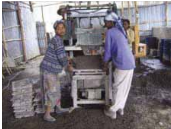
Hollow concrete block production by a small enterprise for housing development in Addis Ababa, Ethiopia.
