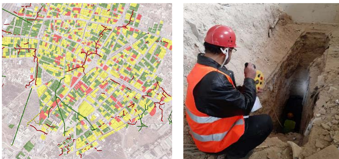
Figure 9 Harasta. Tunnel passing beneath several buildings with depth less than 10 meter from terrain surface. Source: UN-Habitat
