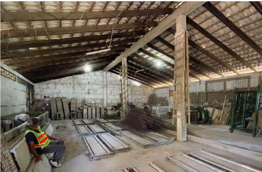
The ferrocement panels are produced locally by L-NGO, allowing for good control of availability and quality
