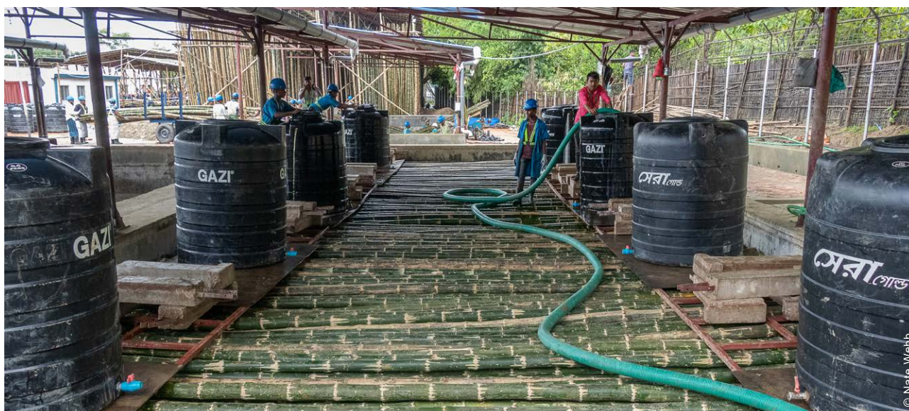
The orthoboric solution used for the treatment of bamboo was selected for its ease in processing and its non-toxic nature.
