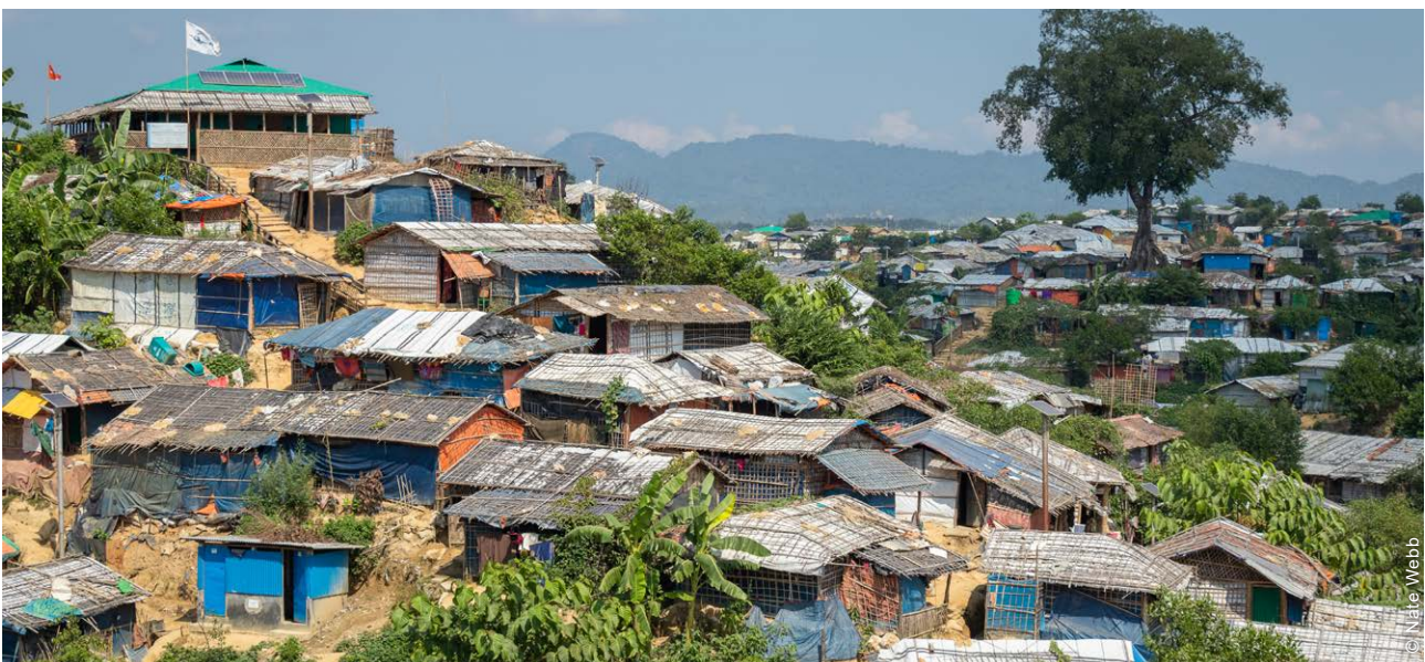
Bamboo is the primary building material in the camps. A GoB policy for non-permanent structures in the camps means that the use of materials such as concrete, brick and steel is restricted.
