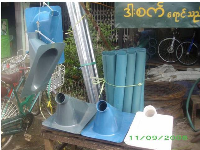
Materials are available locally for latrine construction, including pans and pipes.
