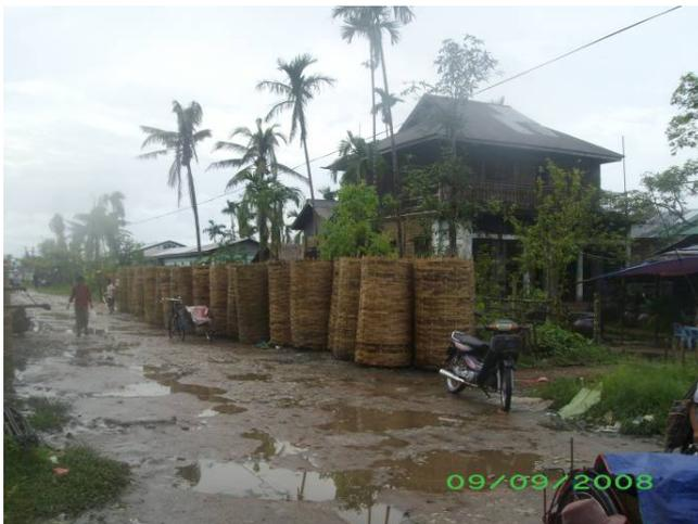
Woven cylinders are manufactured locally to support soakage pits which are important in the construction of latrines.
