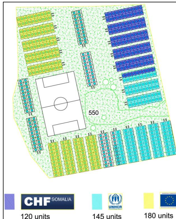
Figure 4: The above diagram is an example of site planning, the distribution of shelters by donor, allowing efficient cost-tracking. UN-HABITAT confirmed that the fire breaks are sufficiently wide to be effective against fire hazards.
